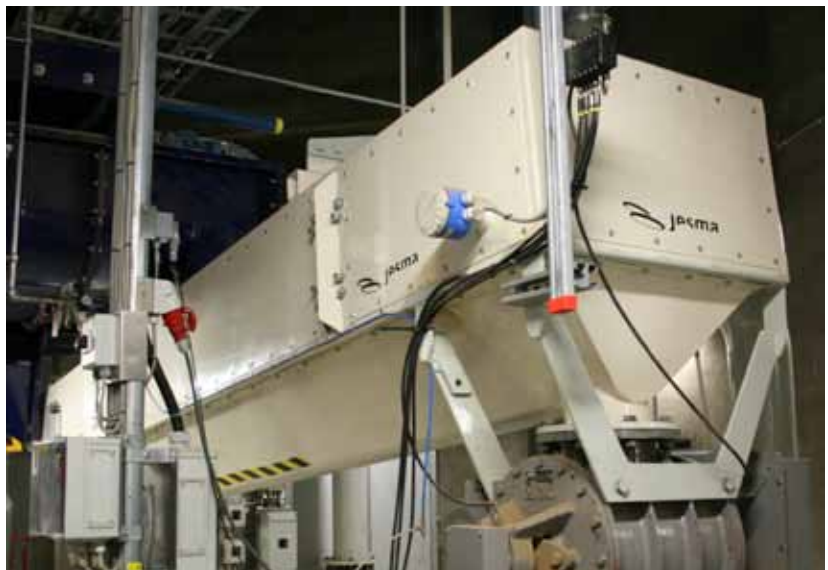
The picture shows the dustproof weigh feeder from Jesma which continuously feeds up to 8 tons of wood pellets per hour.
