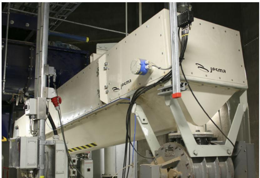
The picture shows the dustproof weigh feeder from Jesma which continuously feeds up to 8 tons of wood pellets per hour.
